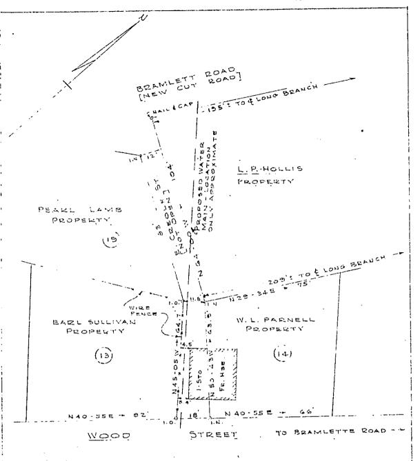
Plat Showing The General Area Where A 5" Water Main is Proposed To Be Constructed Between Bramlette Road and Wood Street, Greenville County, S. C.
